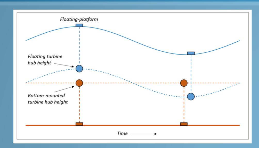
Progressive wave system: Maximum flow asymmetry and hence power asymmetry. Effect is exacerbated for floating devices.
