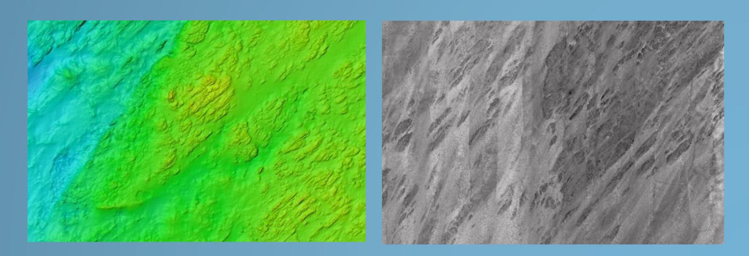
Multibeam echosounders can produce high resolution maps of the seabed. As well as bathymetry, information about the physical composition of the seabed can be derived from the
